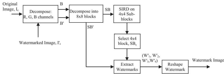
Figure 4. Extraction process.
