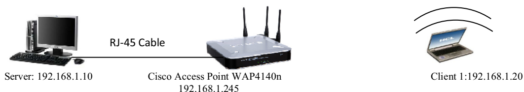
Figure 1 Experimental test-bed design for non-roaming wireless LAN.
