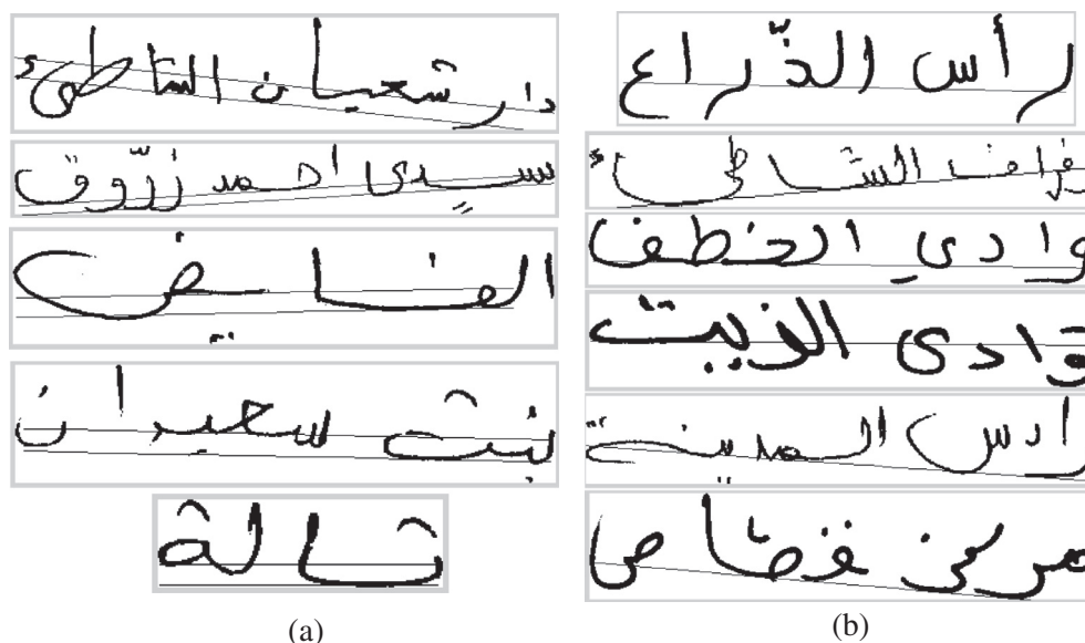
Figure 10 Examples where baselines are maladjusted to the true baseline: (a) examples where subwords have different baselines; (b) examples where one part of city name corresponds perfectly to the true baseline but the remaining part is lying along the lower edge of the isolated characters.
