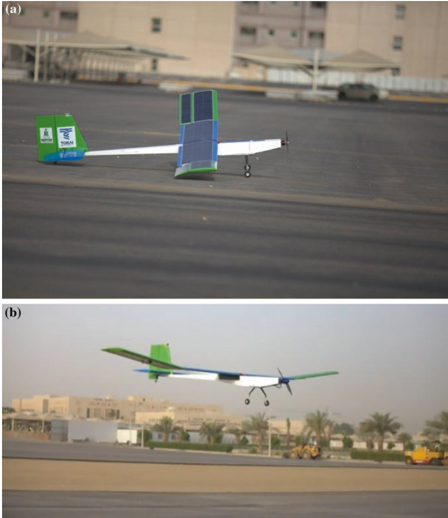
Fig. 7 shows the ‘Solar Falcon-1’ drone. a ‘Solar Falcon-1’ on the ground. b ‘Solar Falcon-1’ in flight above the university buildings
