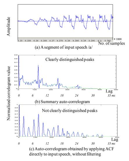
Fig. 3. Illustration of advantage of using summary auto-correlogram, spanned over several filter, rather than using ACF directly on input speech without filtering. The label of horizontal axis corresponds both to lag number (0 100 200 300 400 500) and time (in ms).
