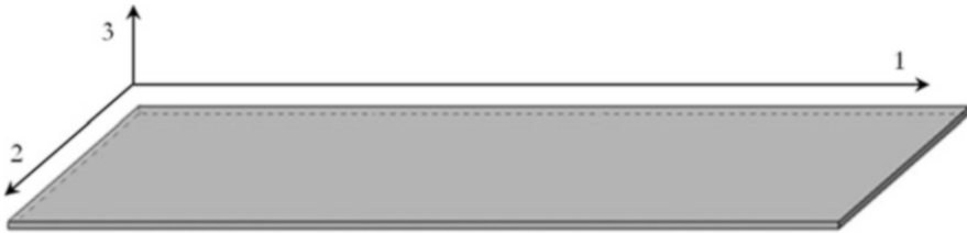
Fig. 3.7 Coordinates for thin plate-like structure
