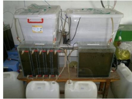
**Fig. 4** Lab-scale ABR and completed mixed anaerobic reactor in operation.
