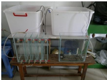
**Fig 3** Lab-scale ABR and completed mixed anaerobic reactor before operating.
